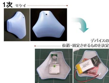
Fig.5 Built-in Device
