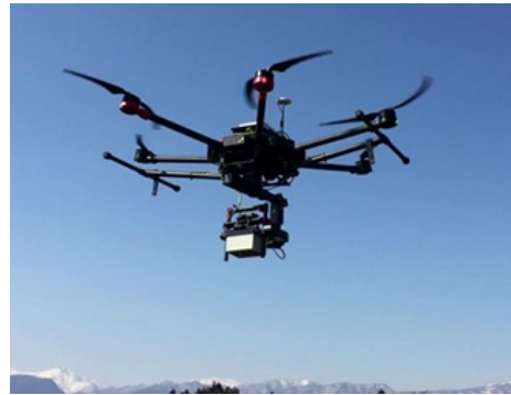
Fig. 2. Matrice 600 [15] equipped with LD-MRS.
